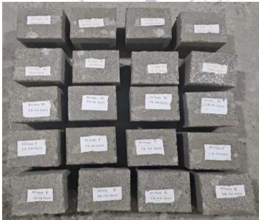
3-rasm. B30(M400) sinfli betonning 10x10x10 namunalari
