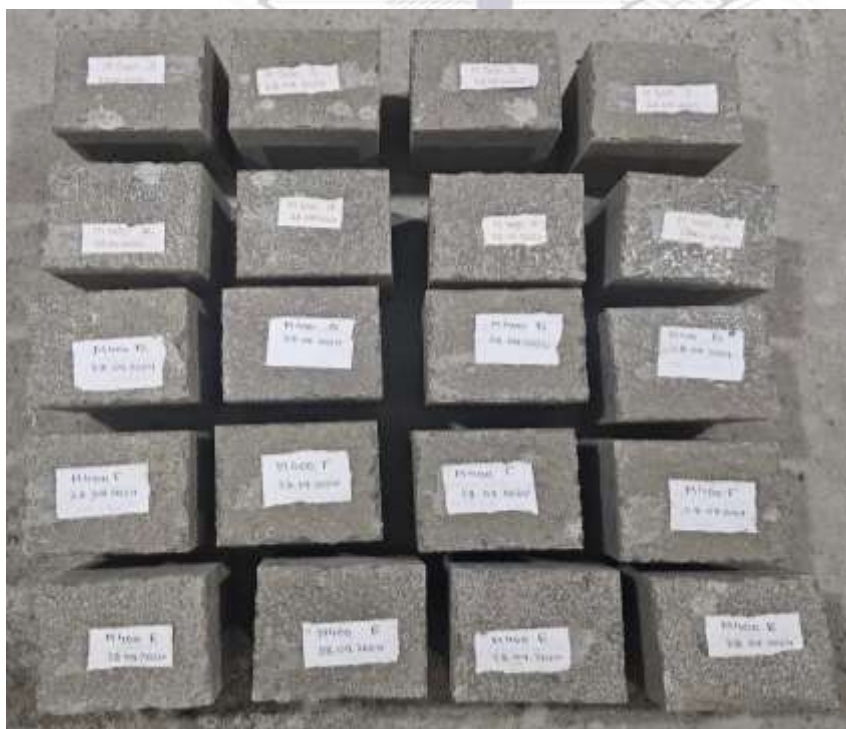
3-rasm. B30(M400) sinfli betonning 10x10x10 namunalari
